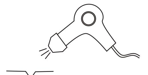
If you find that the rubber is deformed, gently warm the rubber with a hairdrier. But be careful not to overheat the rubber. A gentle heat is all that is needed.
